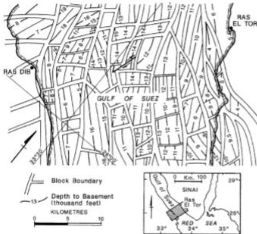
Fig. 35. A detail of the structural map of the Palaeozoic basement of the Gulf of Suez. Contour lines show depth to basement in thousand feet. (After Hammouda 1986).
