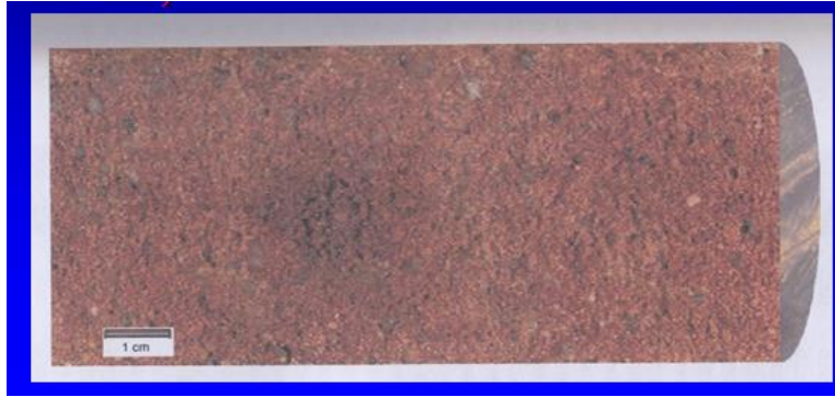
Fig. 46b. Turbidite sandstone core from Campos Basin, Brazil (From: Grochau & Gurevich, Geophysics 73(2)2008: E59-E65).
