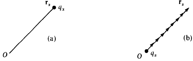
Figure 3.1: Illustration of the Power form of the polarization field for a single point charge reproduced from Cohen-Tannoudji et al. (1997) p. 281. The real charge distribution (a) is a point charge q_\alpha at \mathbf{r}_\alpha . It is equivalent (b) with the reference charge distribution ( q_\alpha at O ) plus n dipoles q_\alpha \mathbf{r}_\alpha / n . The Power form of the polarization field for this situation is obtained as the limit n \rightarrow \infty .
