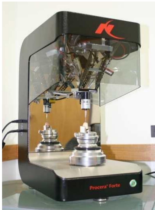
2. ábra A Procera Forte a cég harmadik generációs szkennere. (Abdullah O, Azari A. An introduction to dental digitizers in dentistry; systematic review. Journal of Chemical and Pharmaceutical Research . 10/11 2018;7:10-20.)
