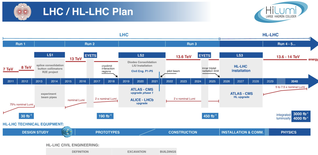
Figure 3.3: The history and the future planning of the LHC project showing the development of the peak collision energy and the delivered luminosity as a function of time, including the High-Luminosity LHC (HL-LHC) era from 2029. While Run 1 started in 2009, the figure only starts at 2011 when luminosity production ramped up. LS stands for long shutdown, EYETS for extended year-end technical stop. During Run 1 the LHC operated with 50 ns bunch spacing, since Run 2 with the design 25 ns.
