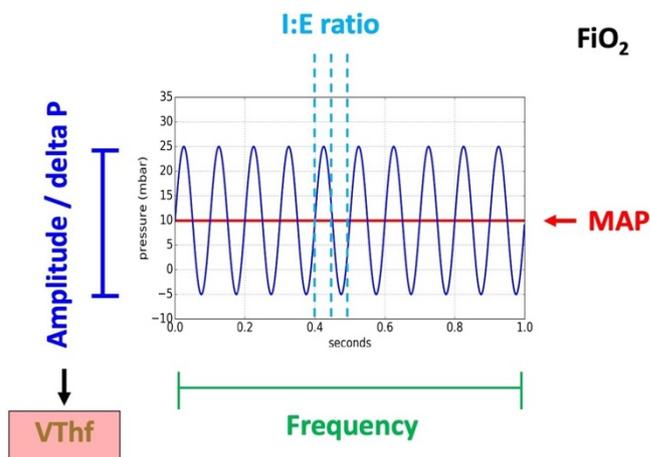
**Figure 15: Ventilator parameters during high frequency oscillatory ventilation (HFOV).** See main text for more details.
